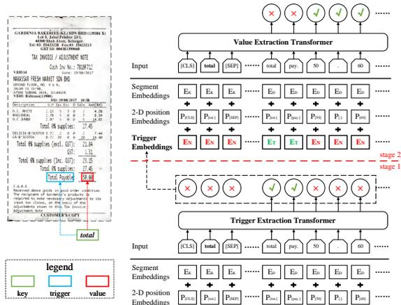
Figure 2: Architecture of the proposed KATA model. The left part presents an example of receipt and the right part presents the trigger extraction module and value extraction module in KATA based on this example.
